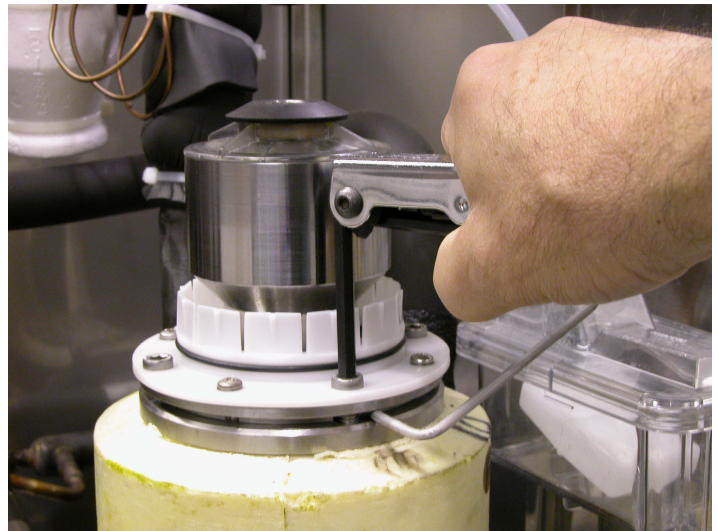
Remove allen head cap screws
